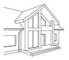
**FOME FLEX HYBRID ROOF&FAÇADE** specifically developed to construction and dilatation joints in façades, roofs and pedestrian walkways on commonly used building materials such as concrete, masonry, painted wood, enamel, aluminium, stainless steel and various plastics.
