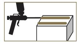
Correction time 2 minutes. The corners of the walls are made according to the instructions of the block manufacturer. Jumpers are laid according to generally accepted installation methods. Application temperature from  $-5^{\circ}$ C to  $+30^{\circ}$ C. If the foam is used at low temperatures, it is necessary to warm the vial to  $+18^{\circ}$ C by placing it in warm water or in a warm room. Uncured foam residue is best cleaned with Fome Flex Foam Cleaner. Remove cured foam mechanically.
